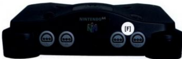
[F] SINCE THE N64 HAS THE HARDWARE TO HANDLE FOUR PLAYER, SPLIT-SCREEN GAMES LIKE MARIO KART 64 NINTENDO THOUGHTFULLY ENGINEERED FOUR CONTROLLER PORTS. NO NEED FOR AN EXPENSIVE MULTI-PLAYER ADAPTOR. THE PORTS CAN ALSO BE USED TO PLUG IN OTHER EXPANSION HARDWARE.
