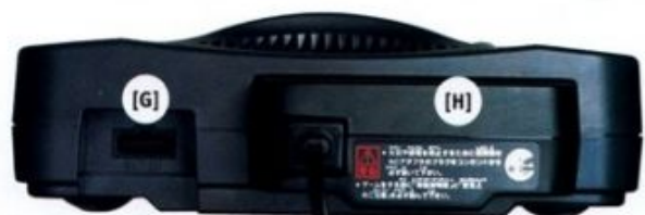
[H] THE N64'S POWER PACK IS ACTUALLY A LARGE REMOVABLE BLOCK, SIMPLIFYING MANUFACTURING OF N64'S FOR DIFFERENT COUNTRIES. [G] NINTENDO'S PATENTED A/V OUTPUT ALLOWS FOR THE CONNECTION OF A WIDE VARIETY OF NINTENDO LEADS FROM RF CABLES TO SUPER VIDEO AND SCART.
