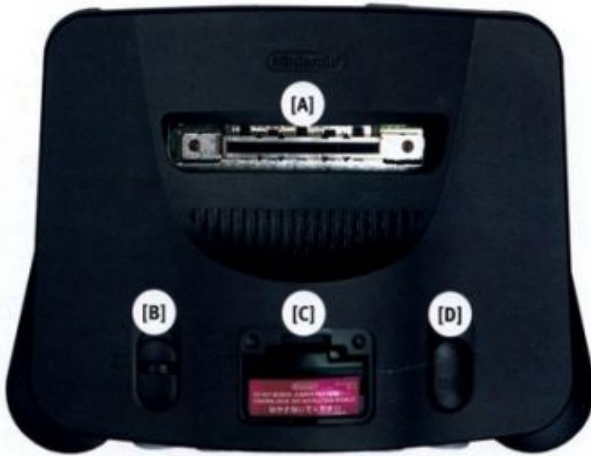
[A] THE CARTRIDGE PORT - THE US N64 USES EASILY REMOVABLE PLASTIC PEGS TO PREVENT JAPANESE CARTRIGES BEING USED. EUROPEAN SYSTEMS WILL ALMOST CERTAINLY USE MORE ELABORATE SOFTWARE PROTECTION. [B] ON/OFF SWITCH. [C] MEMORY JUMPER PAK. [D] RESET SWITCH.
