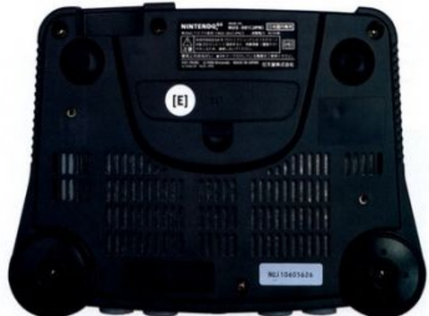
[E] EXPANSION PORT. THE 64DD ADD-ON WILL CONNECT TO THE N64 HERE. ALTHOUGH ITS ACCESS SPEED IS A LOT FASTER THAN A PLAYSTATION'S CD-ROM DRIVE, THE 64DD WILL COME WITH AN ADDITIONAL 2-4MB OF MEMORY TO BUFFER DATA TRANSFERS. THIS MEMORY REPLACES THE MEMORY JUMPER PAK [C].
